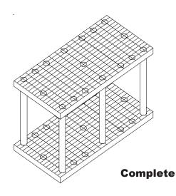
Step 2 Next, slide (1) Top Panel (closed hole sockets) on 36" legs. Make sure panel is pushed all the way down.
