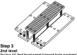
Position (1) 2nd level panel (closed hole sockets) on (6) 24" legs located in floor panel. Insert legs into outside sockets of 2nd level panel. Push down until leg rests on top of socket.
