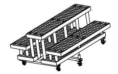
**Step 6** Lift either end of fixture while holding mobile bar in place. Position the last mobile bar in the center of the fixture inserting the stems into the center outside sockets of the floor panels as shown.
