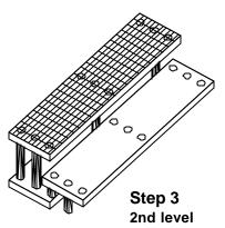
Position the top panel (closed hole sockets) on 24" legs in floor panel overhanging outside edge as shown. (Make sure panels are pushed all the way down.).
