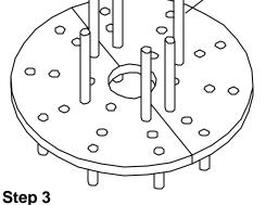
**Bottom Level** Place (6) 36" legs in sockets A,B,C,D,E and F. (Make sure legs go through to ground).
