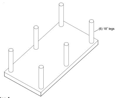
Step 1 Invert panel and place 18" legs as shown. (Make sure legs are pushed all the way down).
