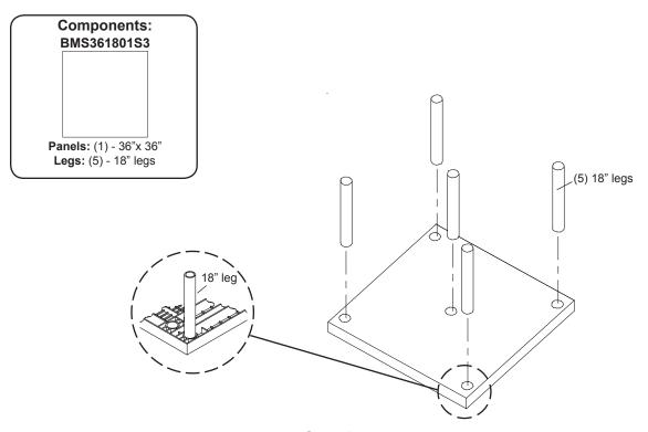
Step 1 Invert panel and place 18" legs as shown. (Make sure legs are pushed all the way down).
